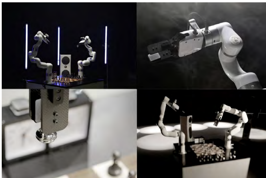
Figure 4: Power Chess (2021) completed system including the sound (upper left speakers), gripper specific for our chess pieces (lower left), 5-axis arm system (upper right), and presentation in dramatic form with chess board in a theatrical setting (lower right).
