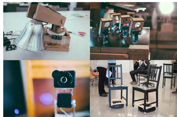
Figure 1: Machines that use gestures to interact with humans. A shy lamp that looks away when humans approach (upper left; LC, 2019). A set of performance micromachines that enact Shakespeare’s Romeo and Juliet when audience is not watching (upper right; LC, 2019). A surveillance camera that follows your face to project it on a face sculpture (lower left; LC et al, 2019). Chair robots that roam in space, making locomotive gestures like “you go first” and “follow me” (lower right, Knight et al, 2017).
